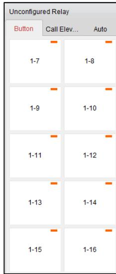
4. Click and drag the unconfigured relay from the Unconfigured Relay panel to the corresponding floor in the Floor List panel.
