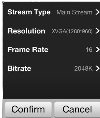
2. Configure the parameters according to actual needs, including Stream Type, Resolution, Frame Rate and Bitrate.
